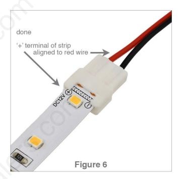
**TIP:** To ease closure of connector cover, one can reduce the thickness of LED strip by removing the paper backing and adhesive for the portion that goes into the connector.
