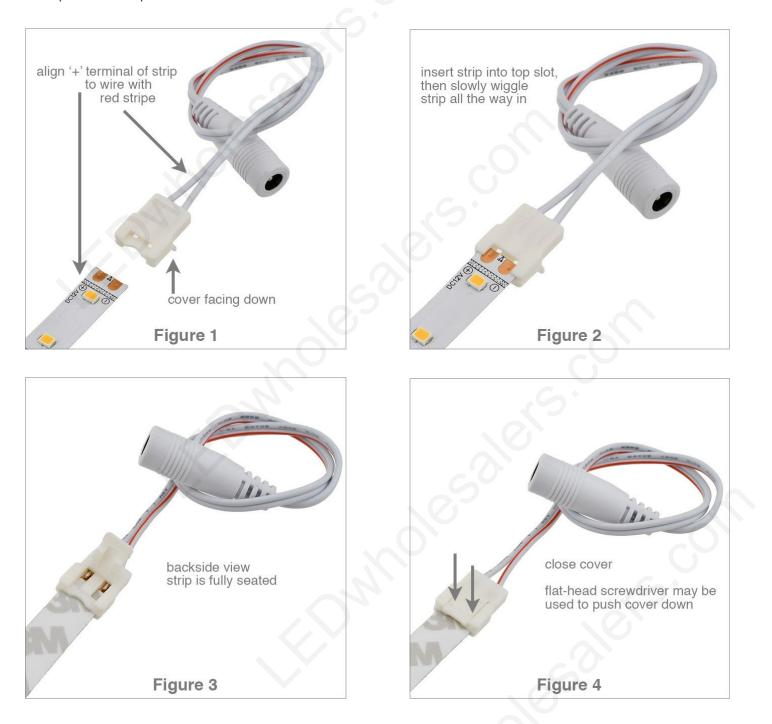
**TIP:** To ease closure of connector cover, one can reduce the thickness of LED strip by removing the paper backing and adhesive for the portion that goes into the connector.
