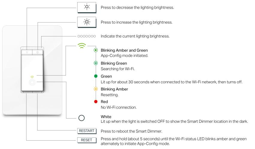
Press and hold (about 10 seconds) until the Wi-Fi status LED blinks amber rapidly to factory reset the Smart Dimmer.
