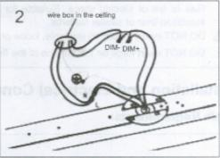
2. Connect AC wire and dimming wire.
