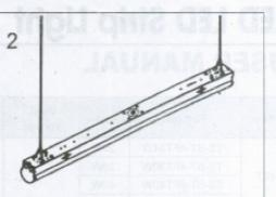
Fix chain to installation location, adjust the height of chain until fixture is balanced.
